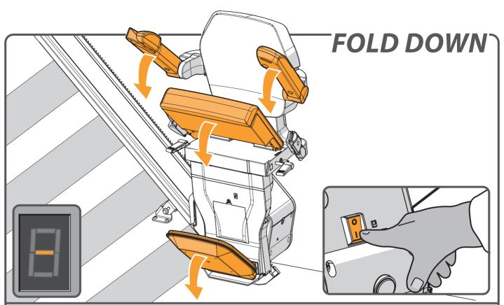
Ensure that the on/off switch is set in the 'ON' position. The diagnosic display will be illuminated when switched on.
