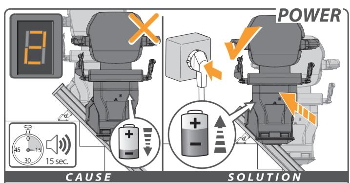
Problem: the lift batteries are not recharging, the lift beeps for 15 seconds and the display shows a "2".
