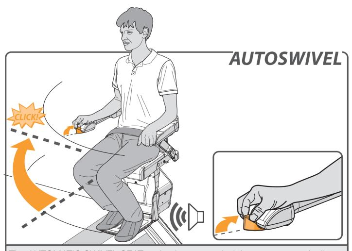
The AUTOMATIC SWIVEL SEAT option lets you swivel the seat automatically to face the direction you are going to walk in. To do this, push and hold the joystick in the direction of travel.
