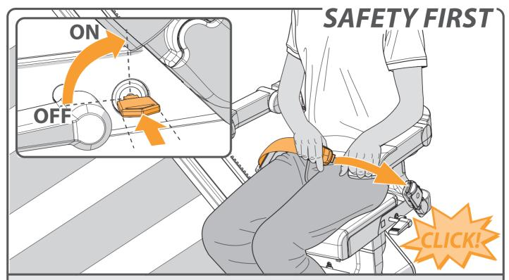
Fasten the seat belt securely, ensuring that it clicks into the holder. Put the key in the switch and turn it ninety degrees clockwise. Check that the chair is in the locked position.
