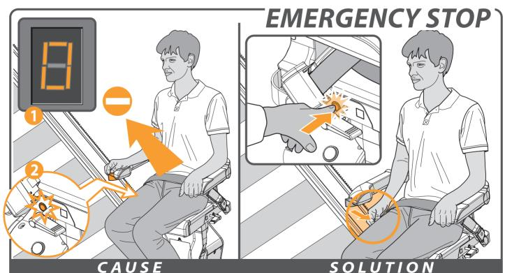
Problem: the lift does not travel in either direction, the display shows a "0" [1]
