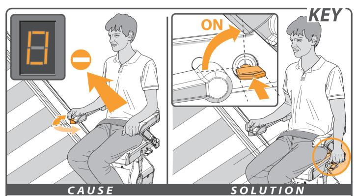
Problem: the lift does not travel in either direction and the display shows a "0".
