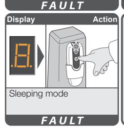
If the display is showing anything but the diagnostic codes listed it requires resetting: drive the lift off the charge contacts. Turn the main switch on the unit unit off for 10 seconds and then back on.
