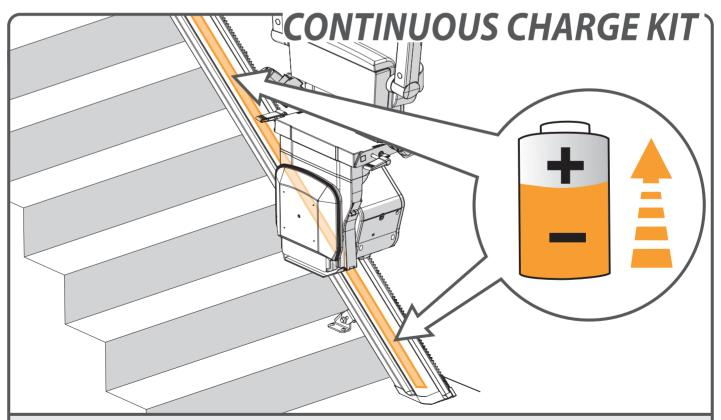
When the CONTINUOUS CHARGE strip is installed, the batteries will charge on every position of the rail.
