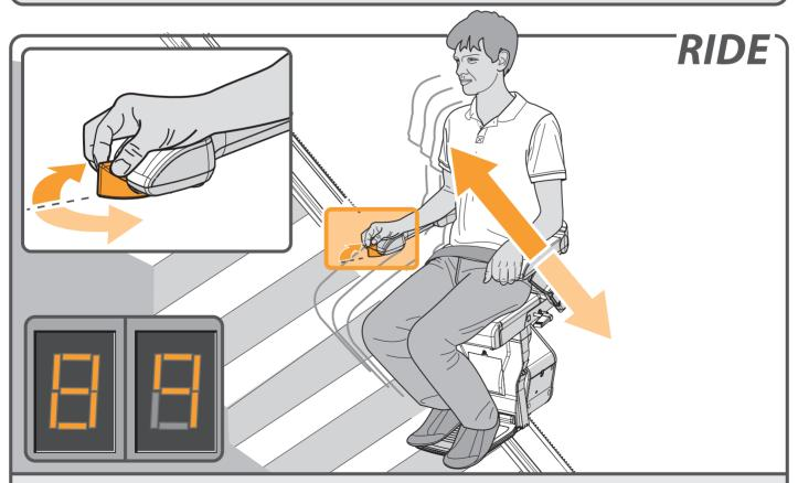
Move the joystick in the desired direction of travel. The display shows a "8/9", the lift gradually starts to move.
