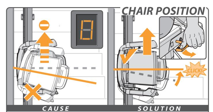
**Problem:** the lift does not travel in either direction and the display shows a "0".
