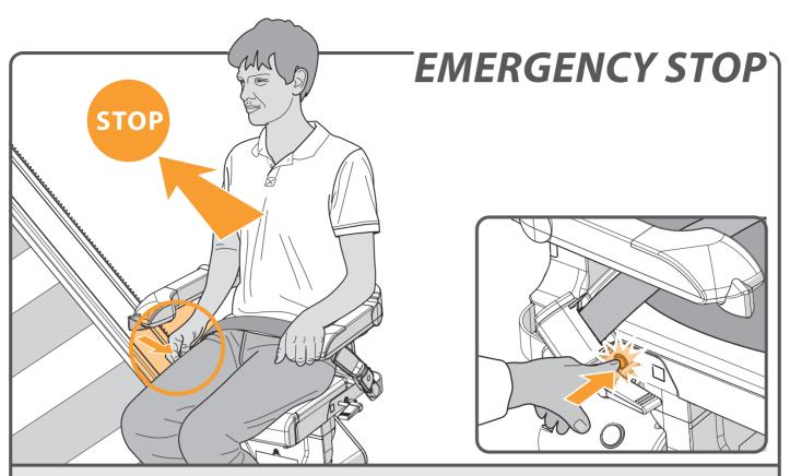
In an emergency, press the emergency stop once. The lift stops straight away. To release the lift, press the emergency stop again.
