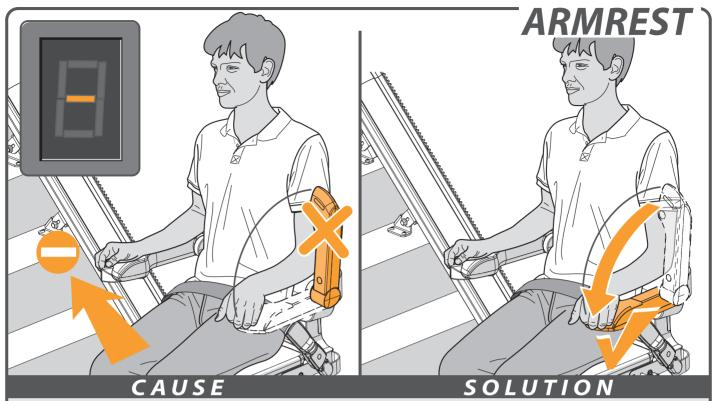
Problem: the lift does not travel in either direction and the display shows a "-".
