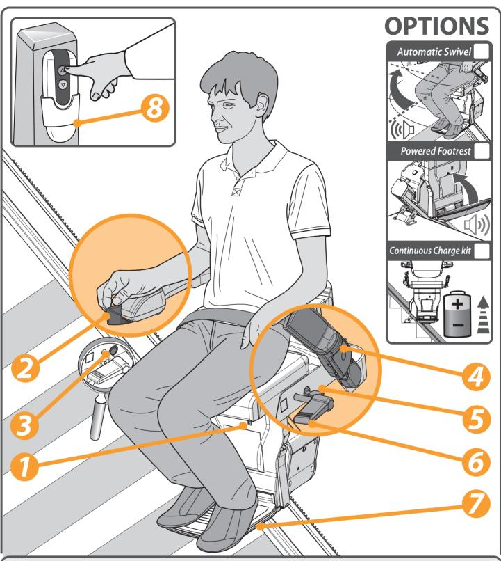
The illustration above shows the features used to operate the XCLUSIVE lift. The XCLUSIVE lift can be upgraded with the Automatic Swivel seat, Powered Footrest and the Continuous Charge kit, options to create even more seat comfort and user-friendliness.
