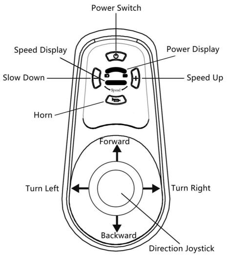
1. Power switch: Press this button to turn on and off the power of the electric wheelchair.
