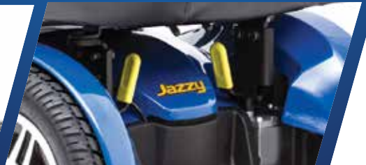
Easy-access free wheel levers
