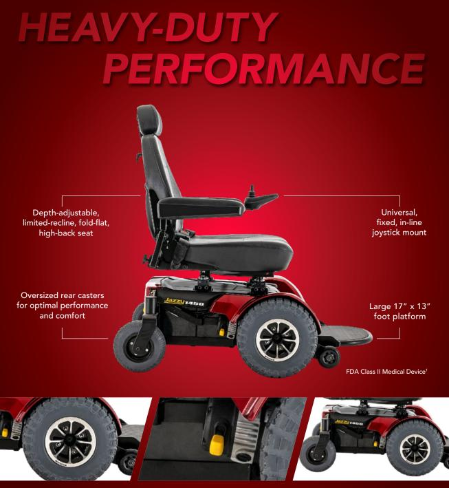
The Jazzy® 14501 offers heavy-duty construction and performance components. This bariatric power chair features a 600 lb. weight capacity, front-wheel drive for superb indoor maneuverability in the tightest of spaces and large front drive wheels for extra absorption over obstacles. The Jazzy 1450 combines superb climbing capabilities with front anti-tips for transitioning over grade changes and handling various terrains easily.
