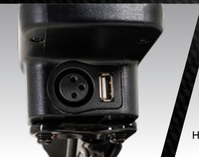
Removable joystick with built in USB charger
