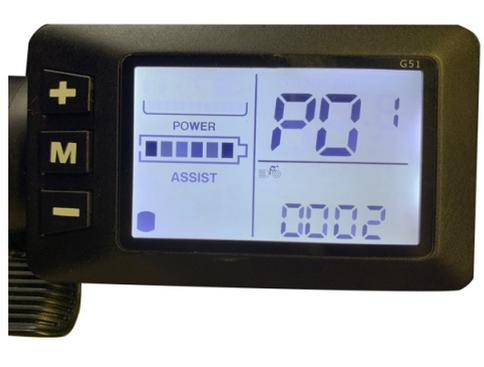
**P01:** Back light Display Brightness - level 1 is the darkest and level 3 is the brightest.
