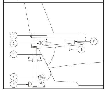
Figure 15. Armrest and Seatback Adjustments
