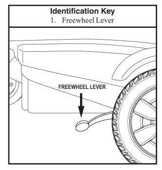
Figure 8. Freewheel Mode (Drive Disengaged)
