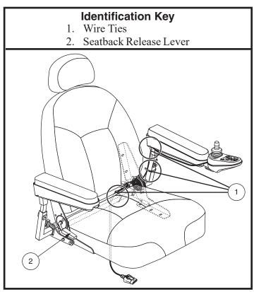
Figure 12. Jazzy Select 6 with Power Seat Controller Routing
