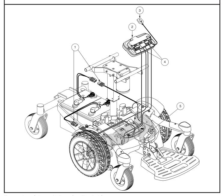
Figure 6. Jazzy Select 6 with Power Seat Electrical Components
