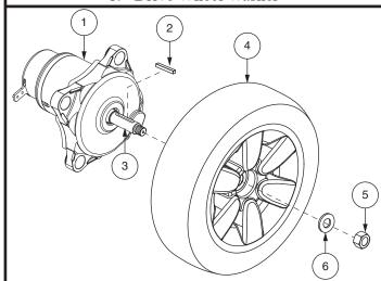
Figure 23. Drive Wheel Removal
