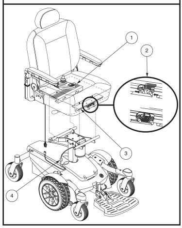
Figure 10. Universal Mounting System on Select 6 with Power Seat
