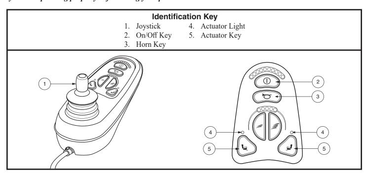
Figure 14. VR2 6-key Controller and Keypad
