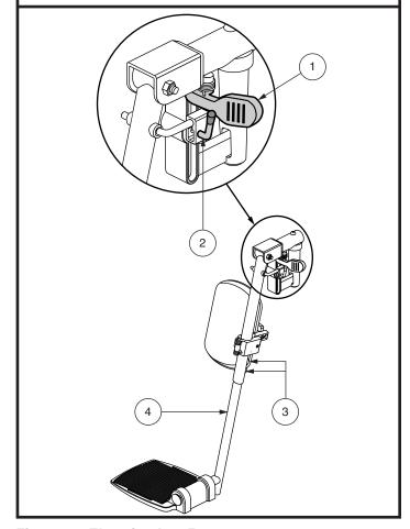
Figure 19. Elevating Leg Rests
