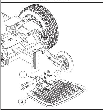
Figure 16. Select Foot Platform Adjustment
