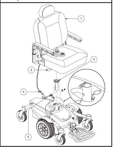
Figure 13. Seat Height Adjustment
