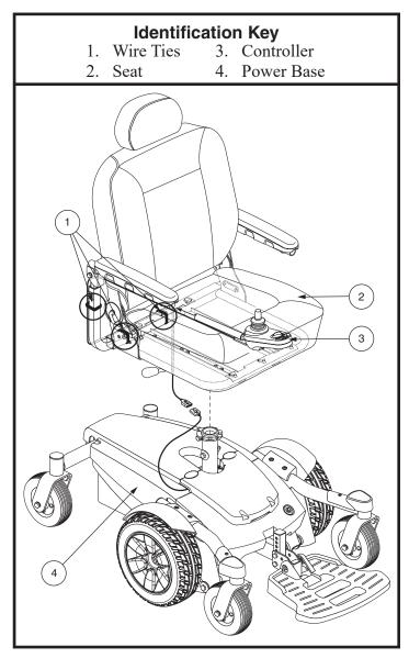
Figure 9. Seat and Controller Assembly
