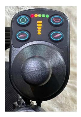
Turning the Matrix **Back Up Beeper** on and off is simple and requires no additional switch.
