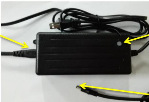
Charger Indicator Light. **Blue** = Connected to Power Source but not charging, it could mean battery is full or battery is not accepting charging. **Green**= Near Full. **Red**=Charging.
