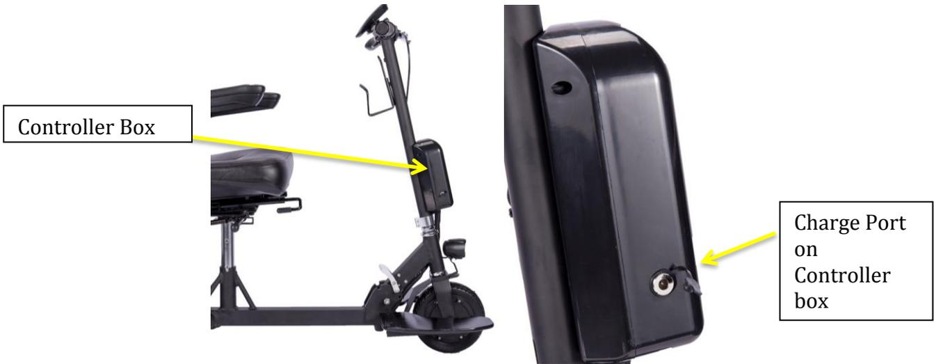
8. Detaching the battery: The battery comes with keys (2) to lock and unlock the battery from the scooter frame. **Please keep the spare key in a safe place. Glion does NOT have replacement keys.** Detach the charging port connector first and then use the key provided to unlock the battery. Slide the battery out of its docking station. You can charge a detached battery using the charge port on the battery.
