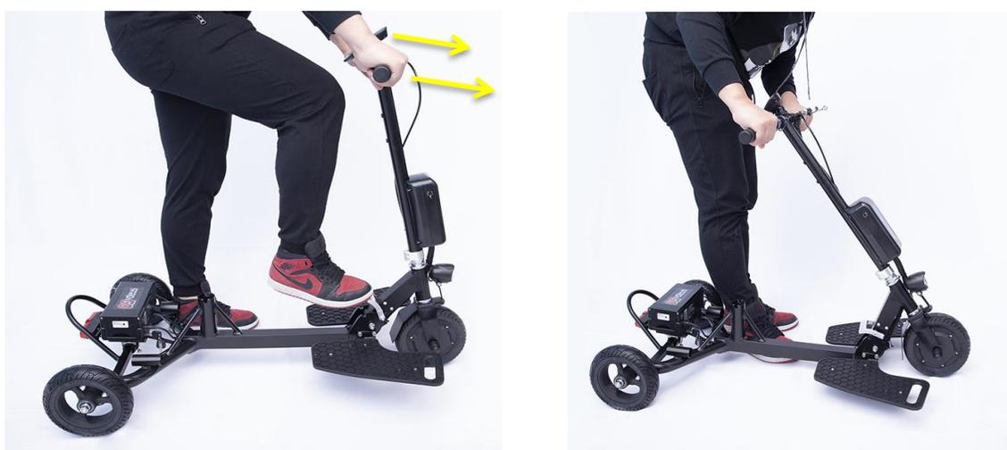
Push T-bar forward to release the pressure on locking mechanism while stepping on the folding lever. **Note: No need to use force from foot, just rest the foot on the folding lever until the handle bar folds down.**
