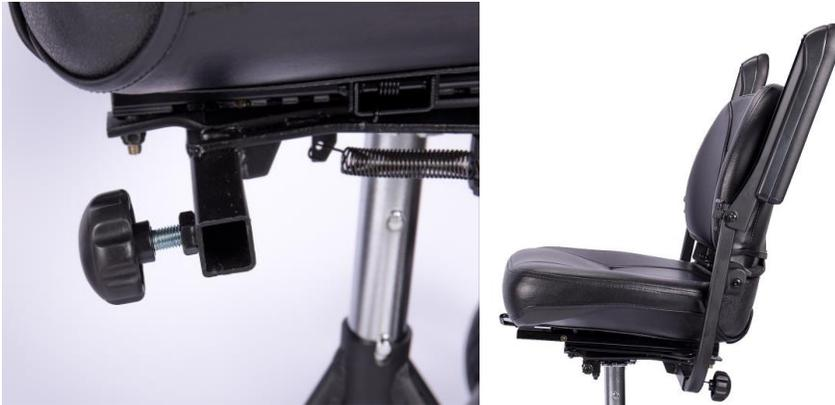
Travel Seat Insert the seat post into the scooter frame. Then insert the travel seat into the seat post.
