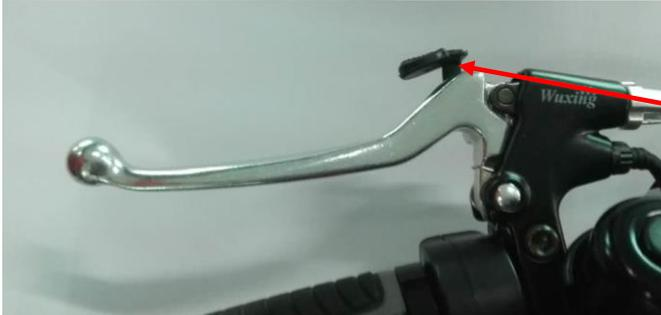
Squeeze the brake handle and push the stopper in. Parking brake is on
