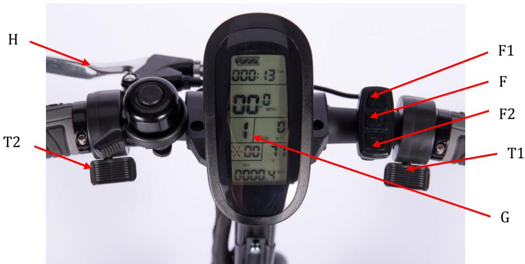
2. **Headlight On/Off:** To turn the headlight on or off, you must first turn on the scooter power (F). While the scooter power is on, press and hold the Gear Up button (F1) for 2 seconds, the headlight and rear light should be turned on. Press and hold (F1) one more time, and the headlight will be turned off.
