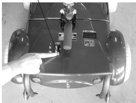
Fig K. Move release bar backward to free wheel mode. (Right motor)
