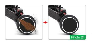
If the Power Wheelchair is on the beach, gravel or wet road, if there is sand, mud or gravel on the tire, it should be cleaned in time to prevent some parts from rusting or the tire running badly, which will affect the beauty and driving comfort and safety (refer to photo 24).
