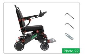
After the Power Wheelchair is used for a period of time, it is necessary to check the screw loosening of the Power Wheelchair to ensure the connection and operation between the parts and components, and to avoid accidents (refer to photo 22).
