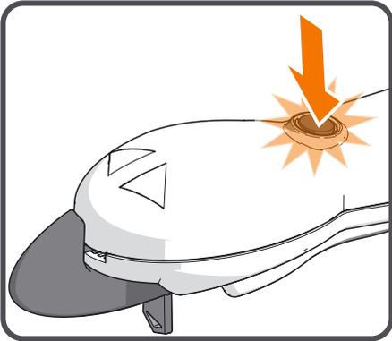
In an emergency, press the stop button once. The lift stops straight away. To release the lift, press the stop button again.
