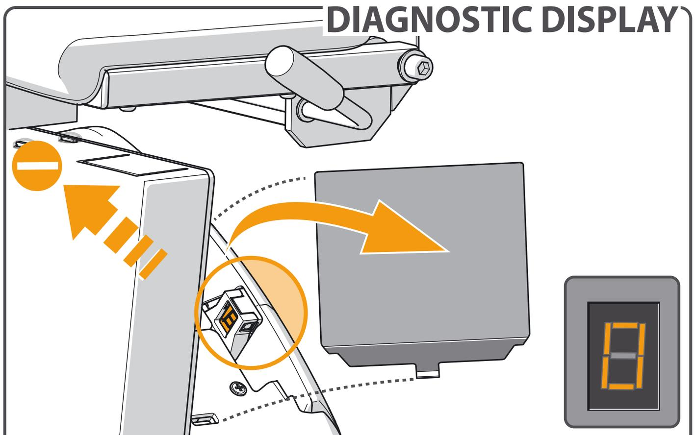
The stairlift is fitted with a diagnostic display that displays a code to help diagnose faults. Refer to APPENDIX {**DIAGNOSTIC CODES**} for an explanation of the diagnostic codes. Please inform the customer service operator of this code when reporting any fault.
