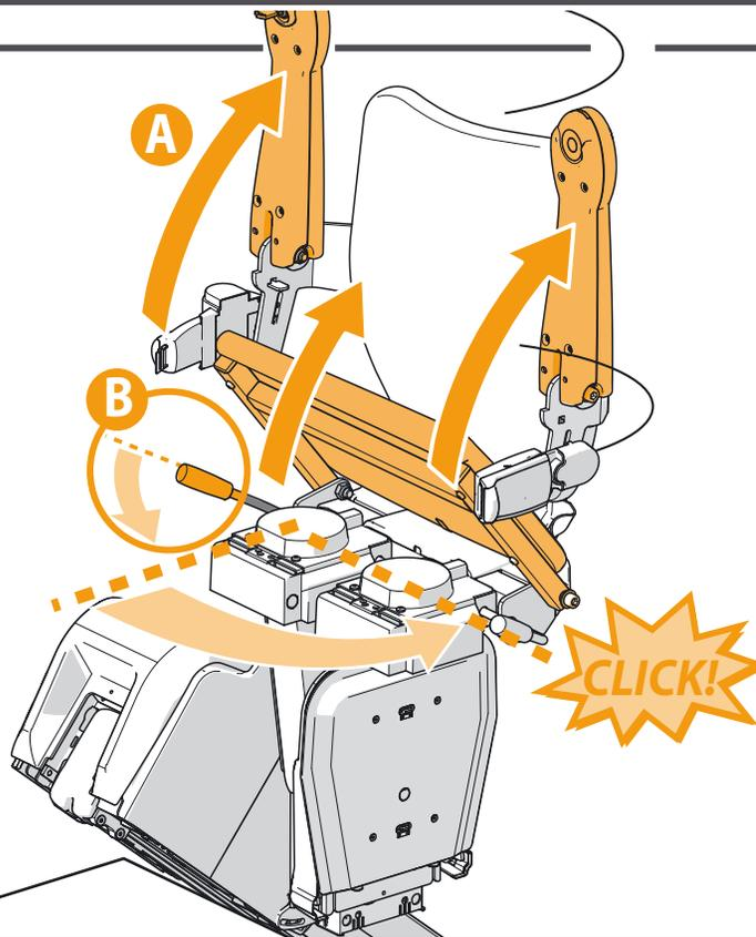
Fold up the armrests and seat {A}. Push the handle, located to the left or right under the seat, downwards {B}. Swivel the seat until you hear a 'click'. The seat is now in the locked position.
