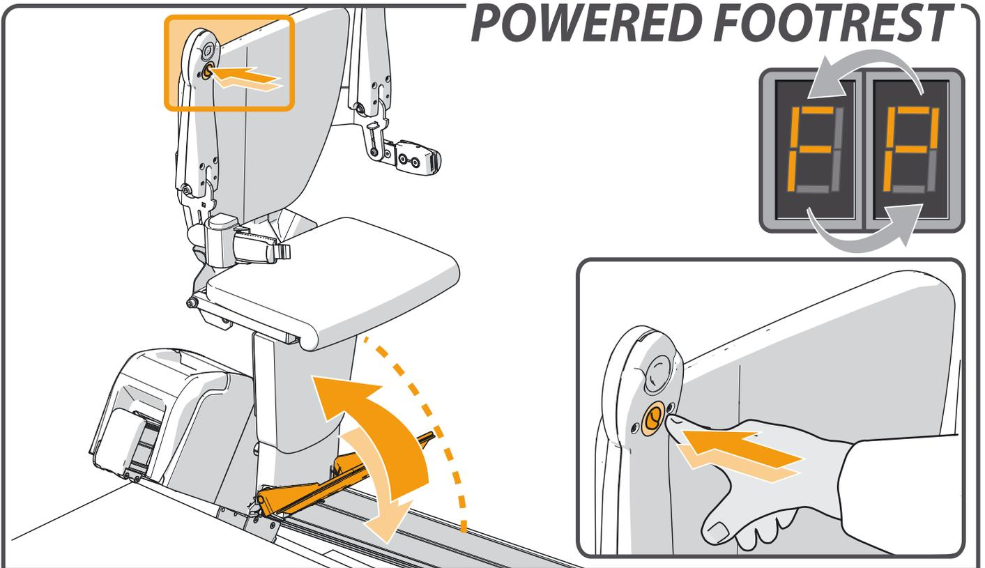
To operate a POWERED FOOTREST press the switch under the armrest. Always ensure the footplate is in the down position during travel.
