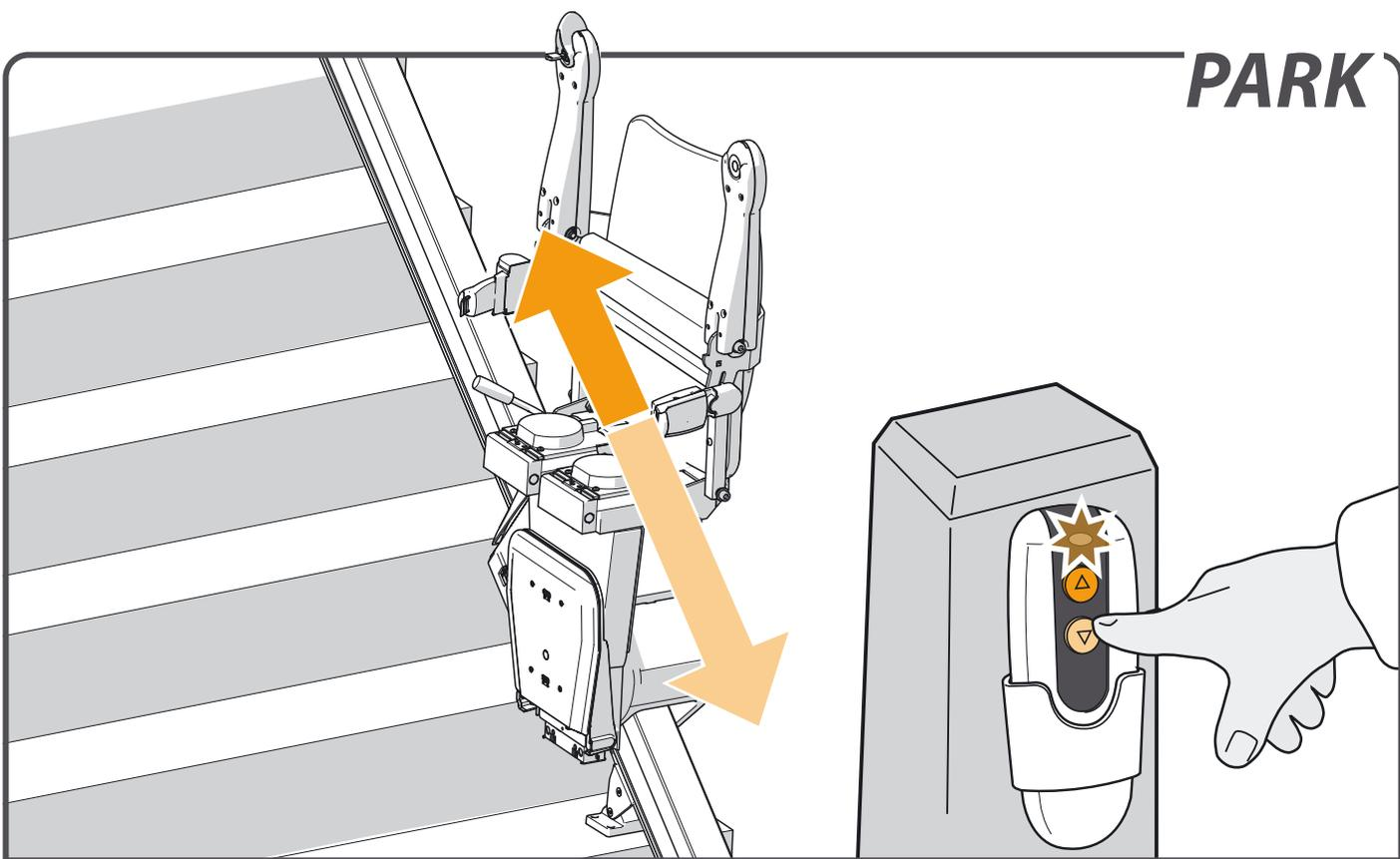
Press and hold the up or down button on the remote control until the lift reaches a stop point. Upon arrival, the lift stops automatically.
