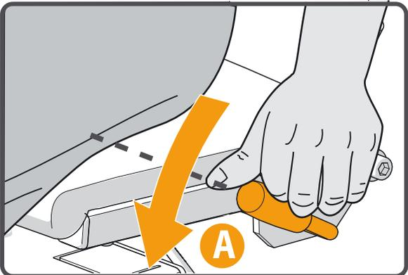
The lift stops automatically at the end of the rail. You should now swivel the seat manually, making it easier to get on and off. To do this, push down the lever{A}. Swivel the seat until you hear a 'click'. The seat is now in the correct position{B}.
